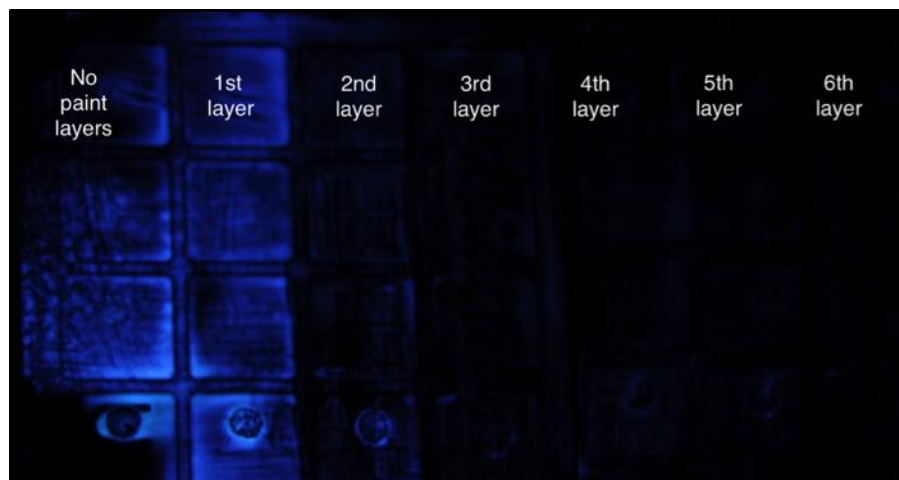
Figure 2. Shows the luminol reaction in the water-based tiles washed when the bloodstains were dried
