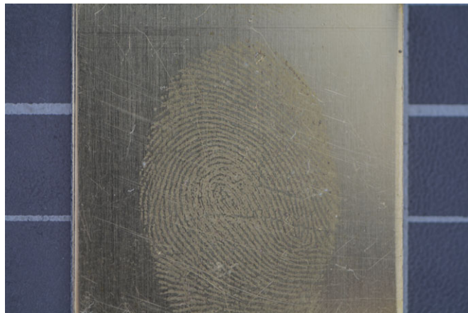
FIG. 2—Fingerprint thermally developed on brass surface.
