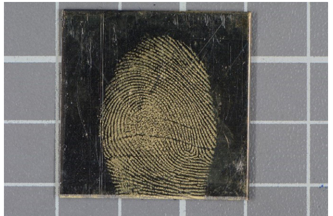
FIG. 6—Fingerprint developed with palladium chloride on brass surface.
