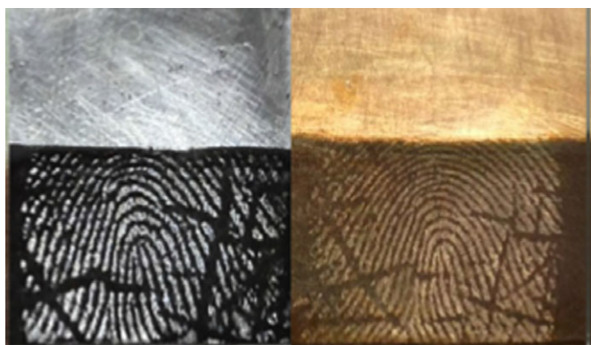
FIG. 11—Electrodeposition of metal nanoparticles on different metal surfaces (left: zinc, right: copper) (64).
