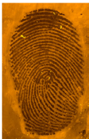
FIG. 8—Fingerprint developed with MMD/ZnO on aluminum foil under 300–400 nm excitation light (58).
