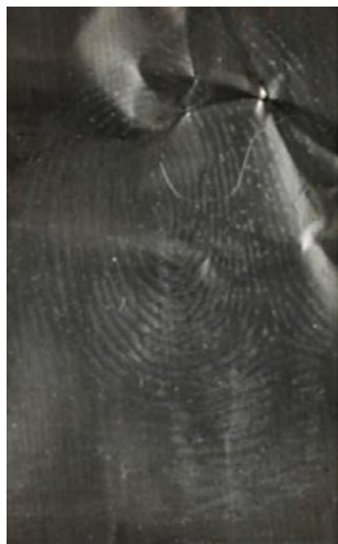
FIG. 9—Fingerprint on aluminum foil developed with single-metal deposition (59).
