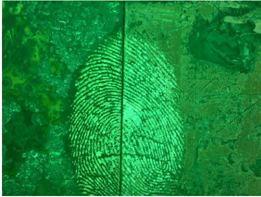
FIG. 4—Fingerprint developed with Lumicyano (left) and normal Cyanoacrylate (right) on brass surface.
