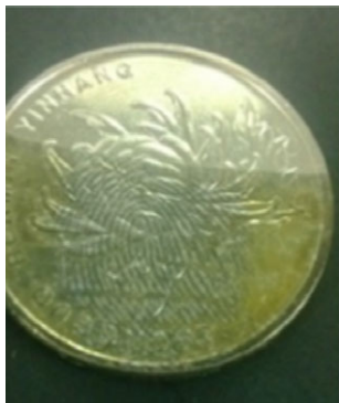
FIG. 10—Fingerprint developed with the electrodeposition of metal nanoparticles method (63).
