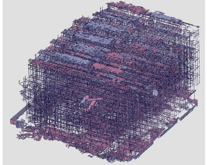
FIG. 4—The Whole 3D scan image of the reconstructed shoring system. The reconstructed 3D shoring system was examined by making cross-section and floor plan drawings.
