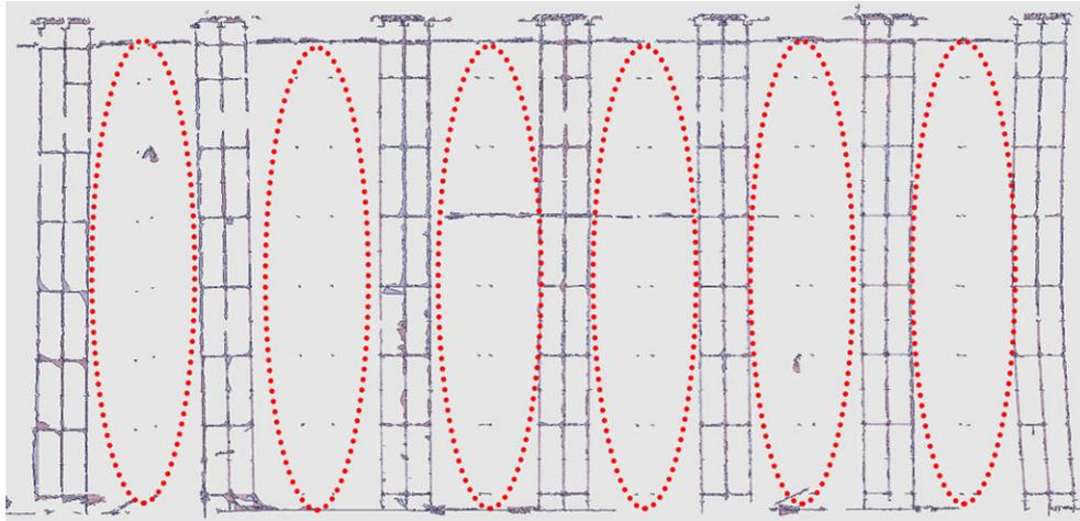
FIG. 6—An example of a cross-sectional drawing of Fig. 4. The dashed circles represent positions where the members were not installed.
