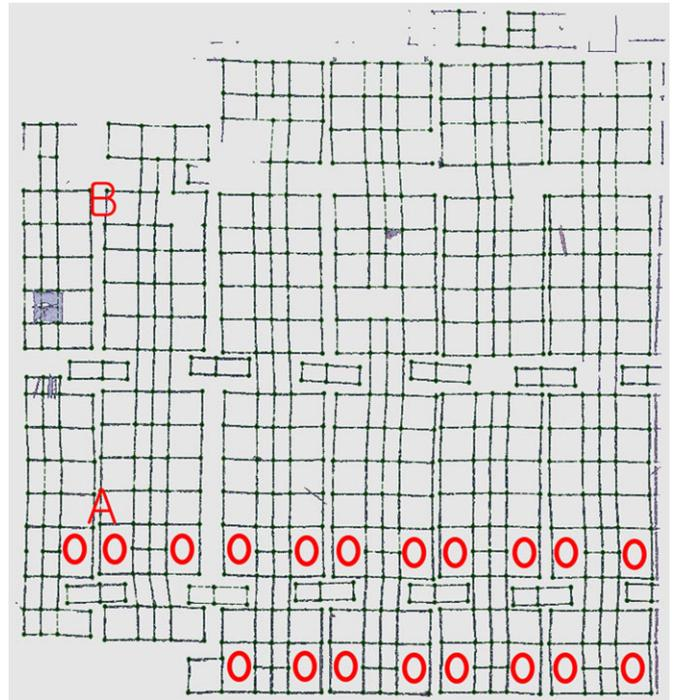
FIG. 5—An example of a floor plan drawing of Fig. 4. The prefabricated shoring system was not installed along the beam so it was not parallel to each other; For example, points A and B and some members shown on the construction drawings were not installed, as indicated by red circles.
